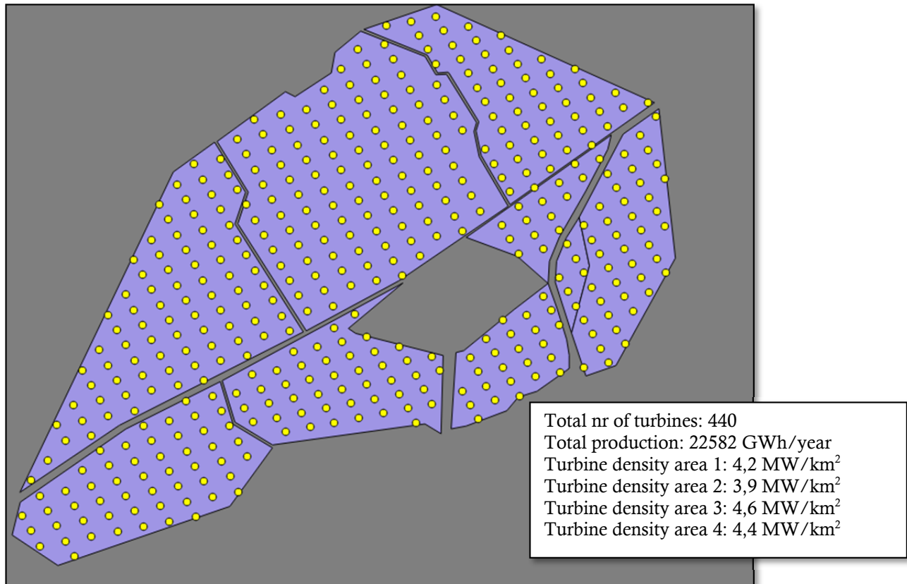
Figure 32: The final layout suggestion using a 10,2:7,1 rotor diameter's spacing in areas 1 and 2, and 9,6:6,7 diameters in area 3 and 4. The layout is rotated -30 degrees from North.
